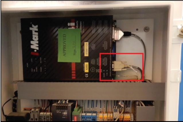
6. Use a compatible hex key to loosen the grommets through which the cables exit each enclosure. Remove the following disconnected cables from the V84i enclosures:
