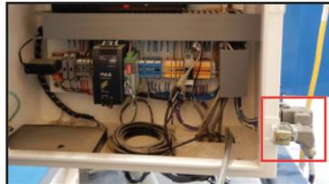
8. Once all cables have been removed, remove any bolts securing the V84i enclosures in place and use a 2-man lift to move the old enclosures clear of the saw.
