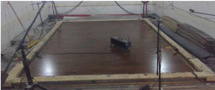
*Photo 1: View of Source Chamber, finish flooring installation observed*
