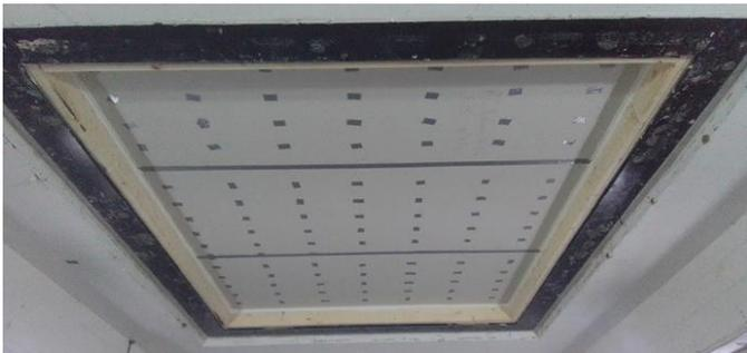
*Photo 2: View of Receive Chamber, bottom of gypsum panel observed*
