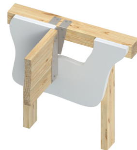
Typical FWHL solid sawn installation (I-Joist similar)
