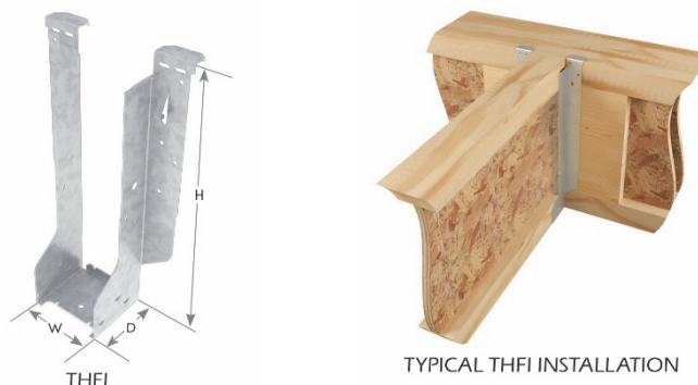
FIGURE 11—THFI FACE MOUNT HANGER
