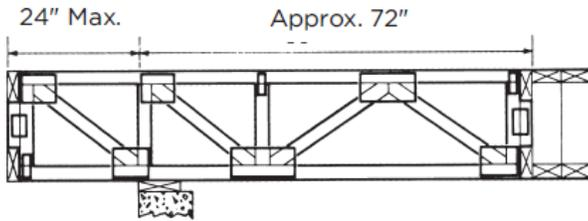
Section AA - Floor Truss Jacks
