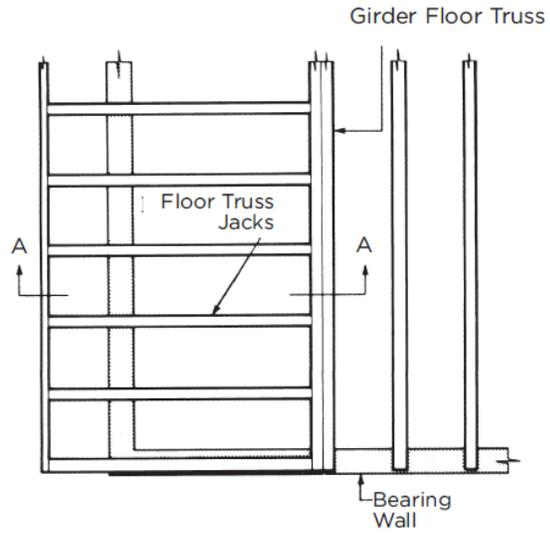
Floor Cantilevered Perpendicular to Floor Truss Span
