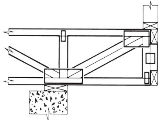
**Load-Bearing Wall Cantilever**
