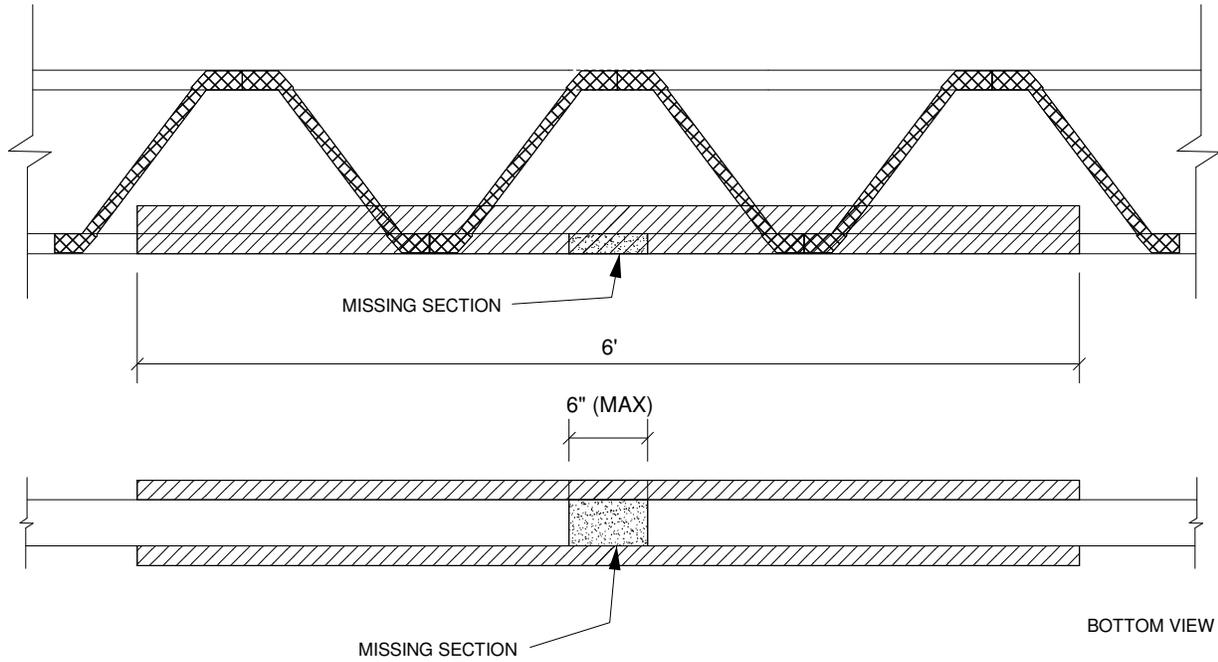
APPLY 2X4X6' SCAB TO BOTH SIDES OF TRUSS CENTERED ON DAMAGE WITH CONSTRUCTION QUALITY ADHESIVE AND 1 ROW OF 10d (0.131" X 3") NAILS SPACED 3" O.C. FROM EACH FACE. SCAB GRADE AND SPECIES TO MATCH EXISTING BOTTOM CHORD.
