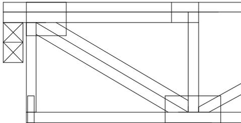
REFER TO INDIVIDUAL TRUSS DESIGN FOR PLATE SIZES AND LUMBER GRADES
