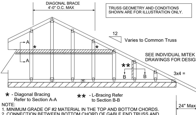
PROVIDE 2x4 BLOCKING BETWEEN THE FIRST TWO TRUSSES AS NOTED. TOENAIL BLOCKING TO TRUSSES WITH (2) - 10d NAILS AT EACH END. ATTACH DIAGONAL BRACE TO BLOCKING WITH (5) - 10d NAILS.
