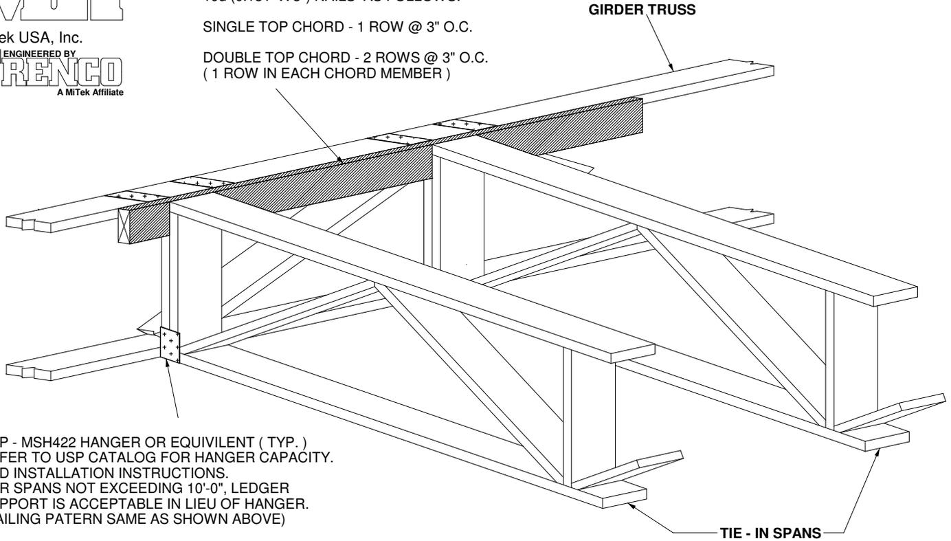
USP - MSH422 HANGER OR EQUIVLENT ( TYP. ) REFER TO USP CATALOG FOR HANGER CAPACITY. AND INSTALLATION INSTRUCTIONS. FOR SPANS NOT EXCEEDING 10'-0", LEDGER SUPPORT IS ACCEPTABLE IN LIEU OF HANGER. (NAILING PATERN SAME AS SHOWN ABOVE)
