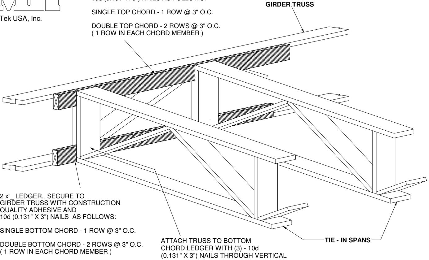
2 x LEDGER. SECURE TO GIRDER TRUSS WITH CONSTRUCTION QUALITY ADHESIVE AND 10d (0.131" X 3") NAILS AS FOLLOWS:
