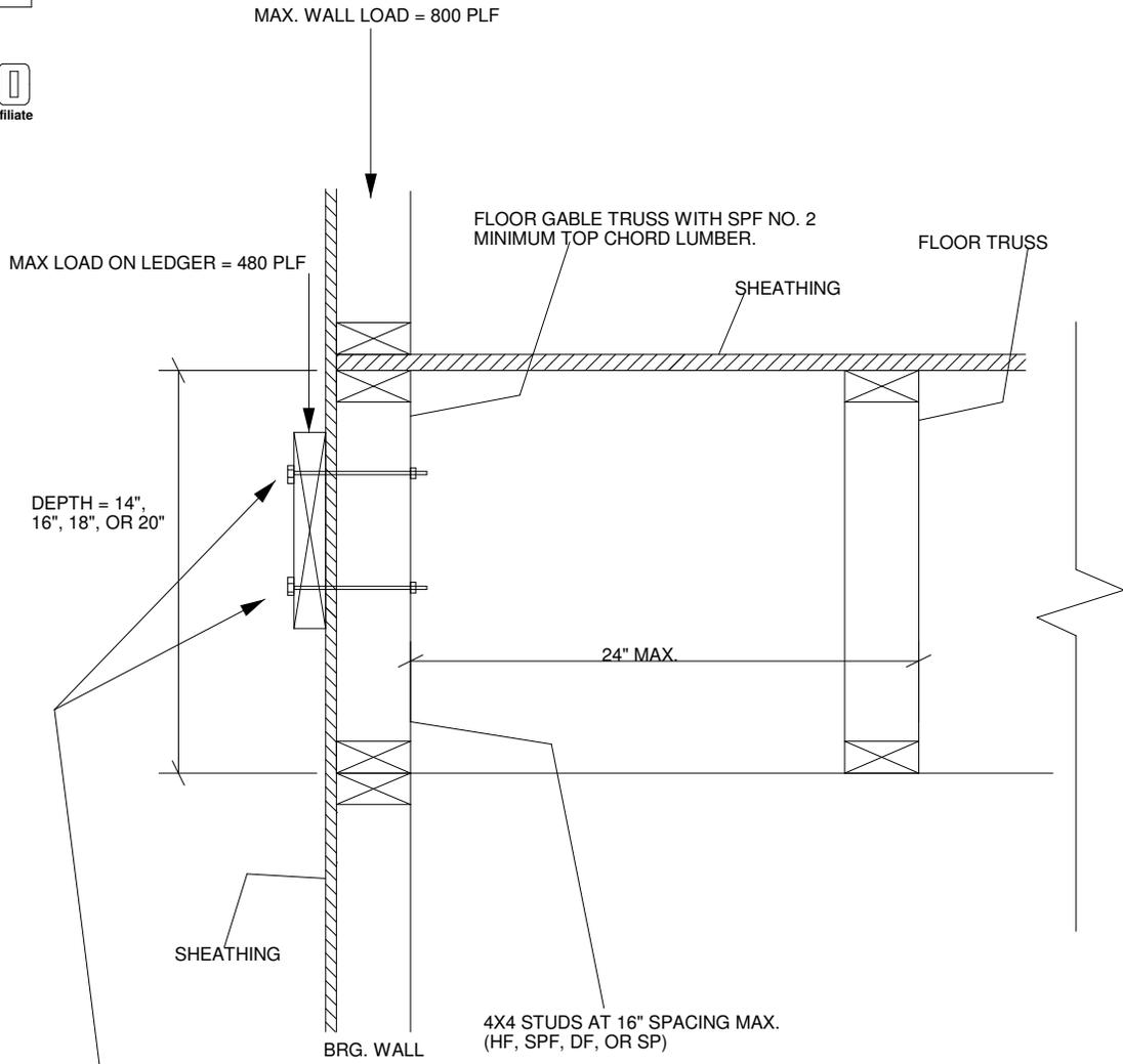
ATTACH LEDGER (DESIGNED BY OTHERS) WITH TWO 1/2" DIAMETER
