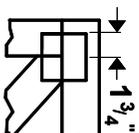
Center plate on joint unless x, y offsets are indicated. Dimensions are in ft.-in.-sixteenths. Apply plates to both sides of truss and fully embed teeth.
