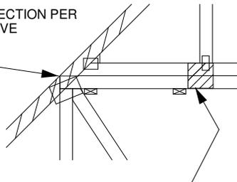
7" x 7" x 1/2" PLYWOOD (or 7/16" OSB) GUSSET EACH SIDE AT 24" O.C. AT EACH BASE TRUSS JOINT. ATTACH WITH 3 - 6d (0.113" X 2") NAILS INTO EACH CHORD FROM EACH SIDE (TOTAL - 12 NAILS)
