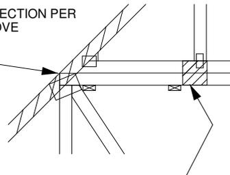
7" x 7" x 1/2" PLYWOOD (or 7/16" OSB) GUSSET EACH SIDE AT 24" O.C. ATTACH WITH 3 - 6d (0.113" X 2") NAILS INTO EACH CHORD FROM EACH SIDE (TOTAL - 12 NAILS)
