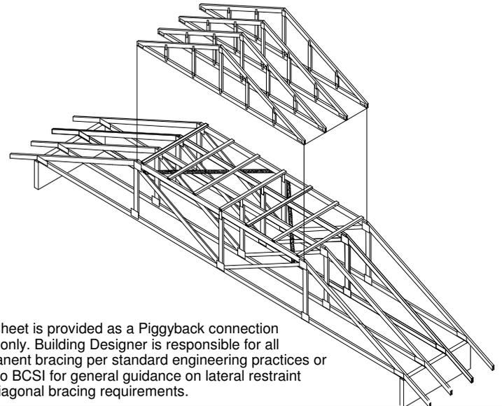
This sheet is provided as a Piggyback connection detail only. Building Designer is responsible for all permanent bracing per standard engineering practices or refer to BCSI for general guidance on lateral restraint and diagonal bracing requirements.
