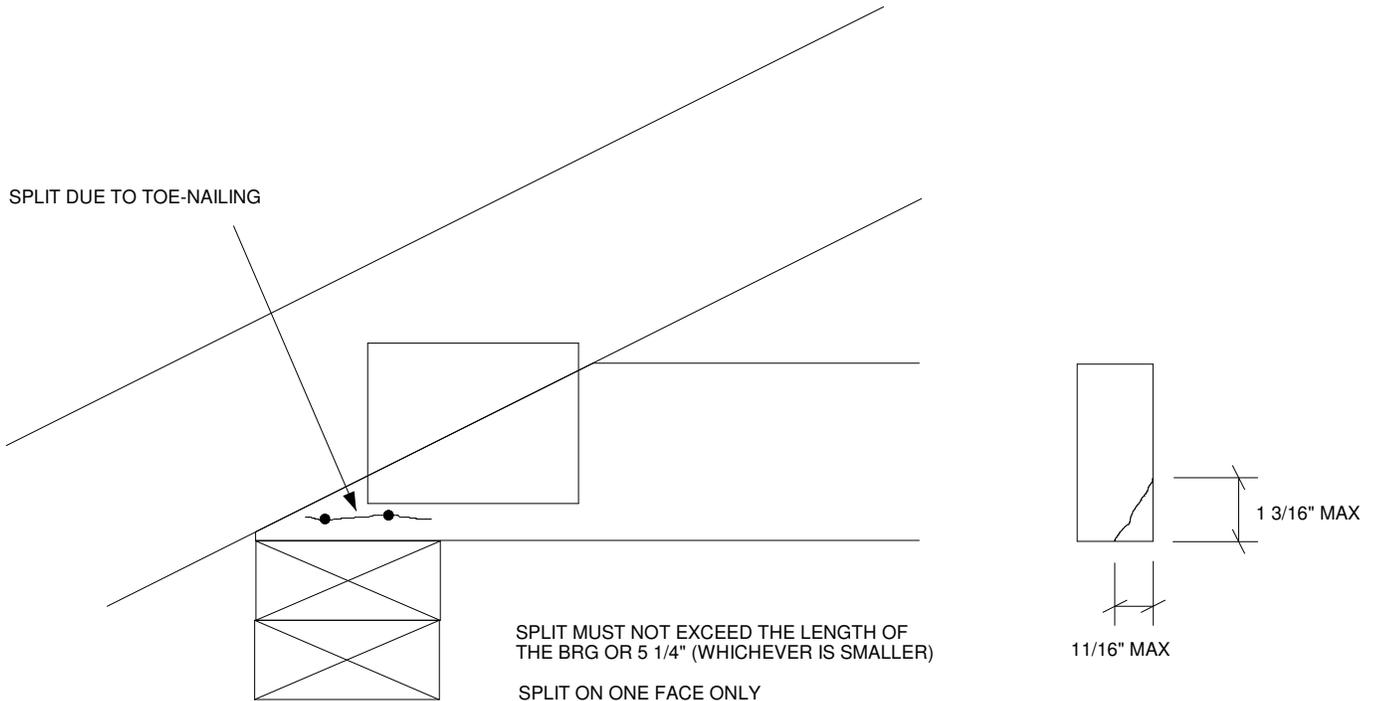
SPLIT MUST NOT EXTEND UNDER CONNECTOR PLATE
