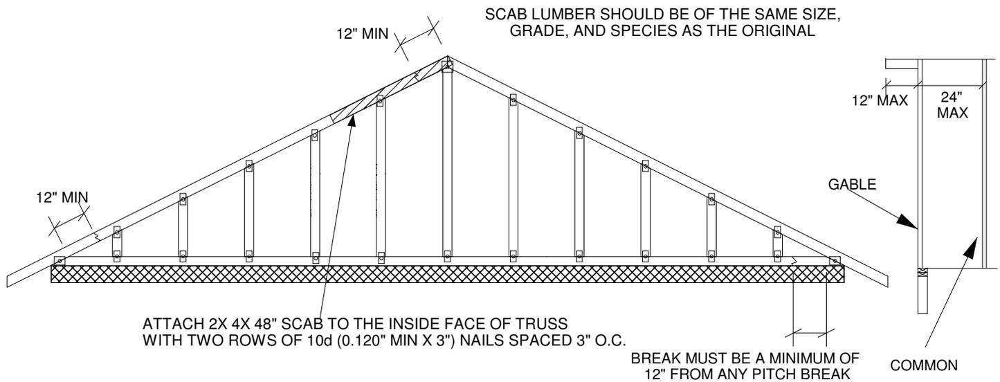
THE OUTSIDE FACE OF THE GABLE MUST BE SHEATHED W/ (MIN) 7/16" O.S.B OR PLYWOOD. SEE MITEK STANDARD GABLE END DETAILS FOR WIND BRACING REQUIREMENTS.
