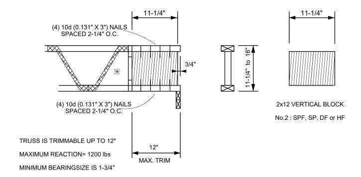
st Last diagonal web must be ran up to the top chord as shown
