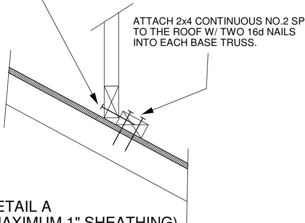
ATTACH 2x4 CONTINUOUS NO.2 SP TO THE ROOF W/ TWO 16d NAILS INTO EACH BASE TRUSS.
