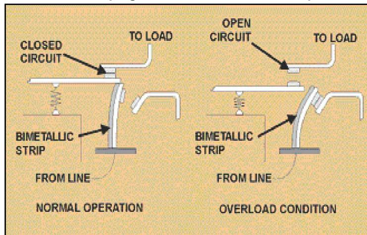
Once the tripping action has taken place, the bimetallic strip cools and reshapes itself, automatically resetting the circuit. The motor can be restarted even when the overload
