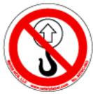
No lift point. Do not lift this device with a hook/crane assembly. Damage to the equipment will be incurred. Refer to the installation instructions.
