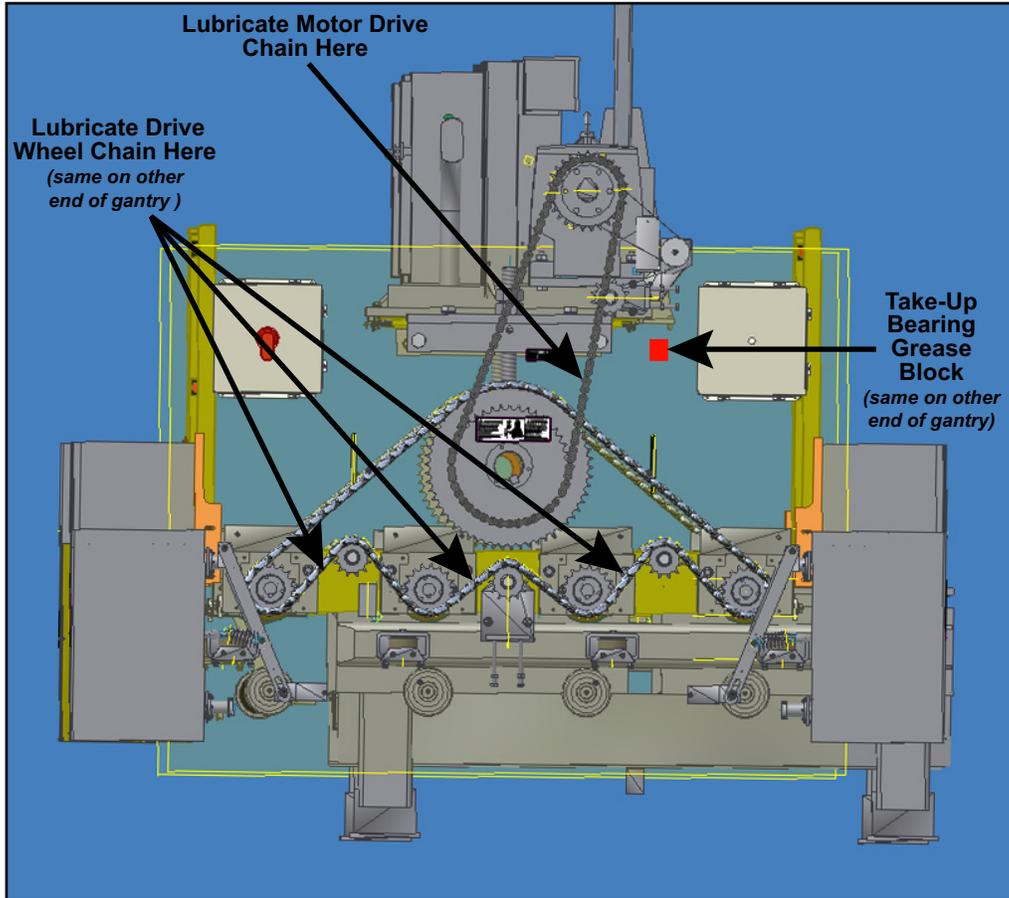
Run the gantry head in the forward (or left) direction after lubricating these points.
