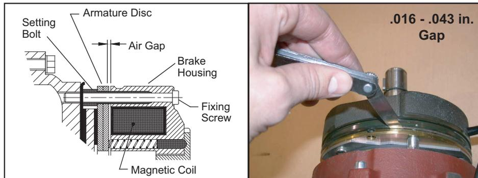
3. If the measurement is outside the allowance recommended at any point around the circumference of the brake, adjust the brake disk air gap using the following steps:
