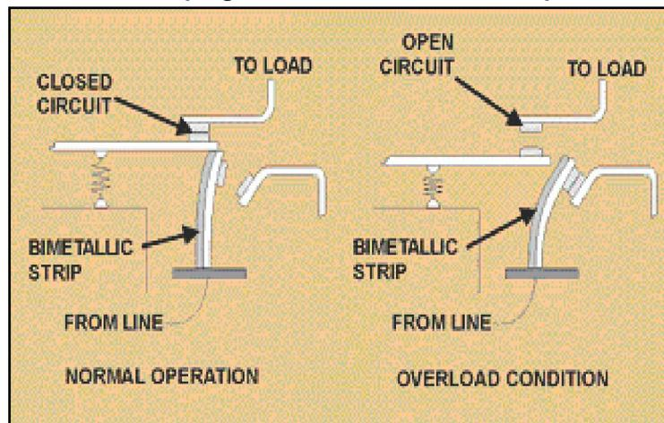
Once the tripping action has taken place, the bimetallic strip cools and reshapes itself, automatically resetting the circuit. The motor can be restarted even when the overload condition has not been cleared, and will trip and reset itself again and again. (This assumes an automatic reset and can also be equipped with a manual reset.)
