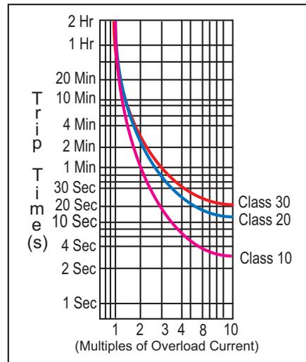
Class 20, and Class 30. Class 10, for example, has to trip the motor off-line in 10 seconds or less at 600% of the full load amps. This is usually sufficient time for the motor to reach full speed.
