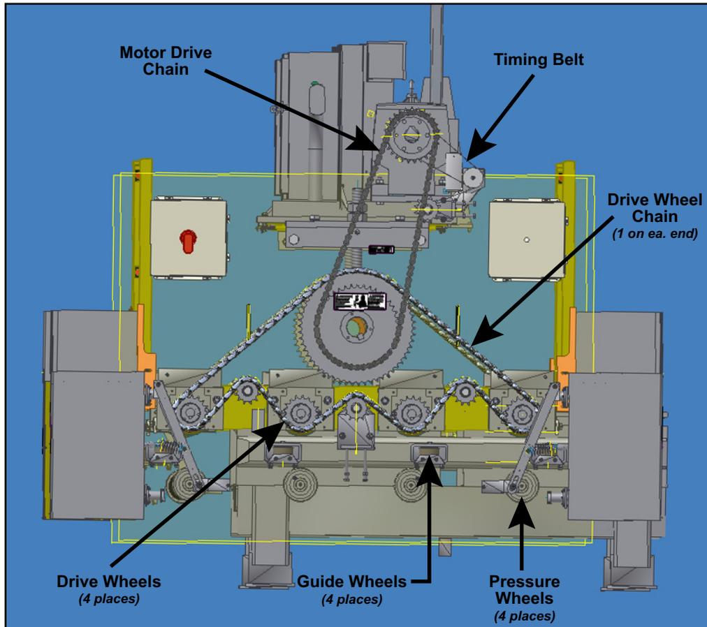
Figure 6-27: Wheels, Chains, and Belt (Machines Shipped After 15 June 2006)
