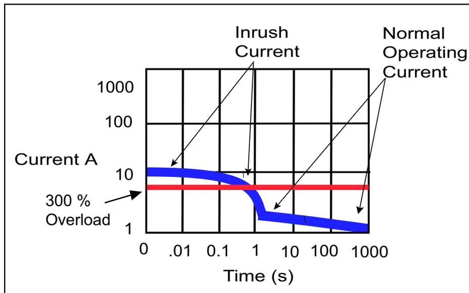
An overload condition will occur when the rotor has difficulty turning and draws more current than it normally would need to keep it turning. When an overload occurs the current being drawn is usually between 2 to 6 times the normal operating current.
