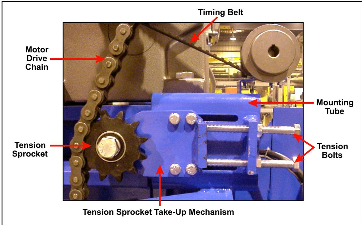
Figure 6-14: Drive Wheel Chain Tensioning
