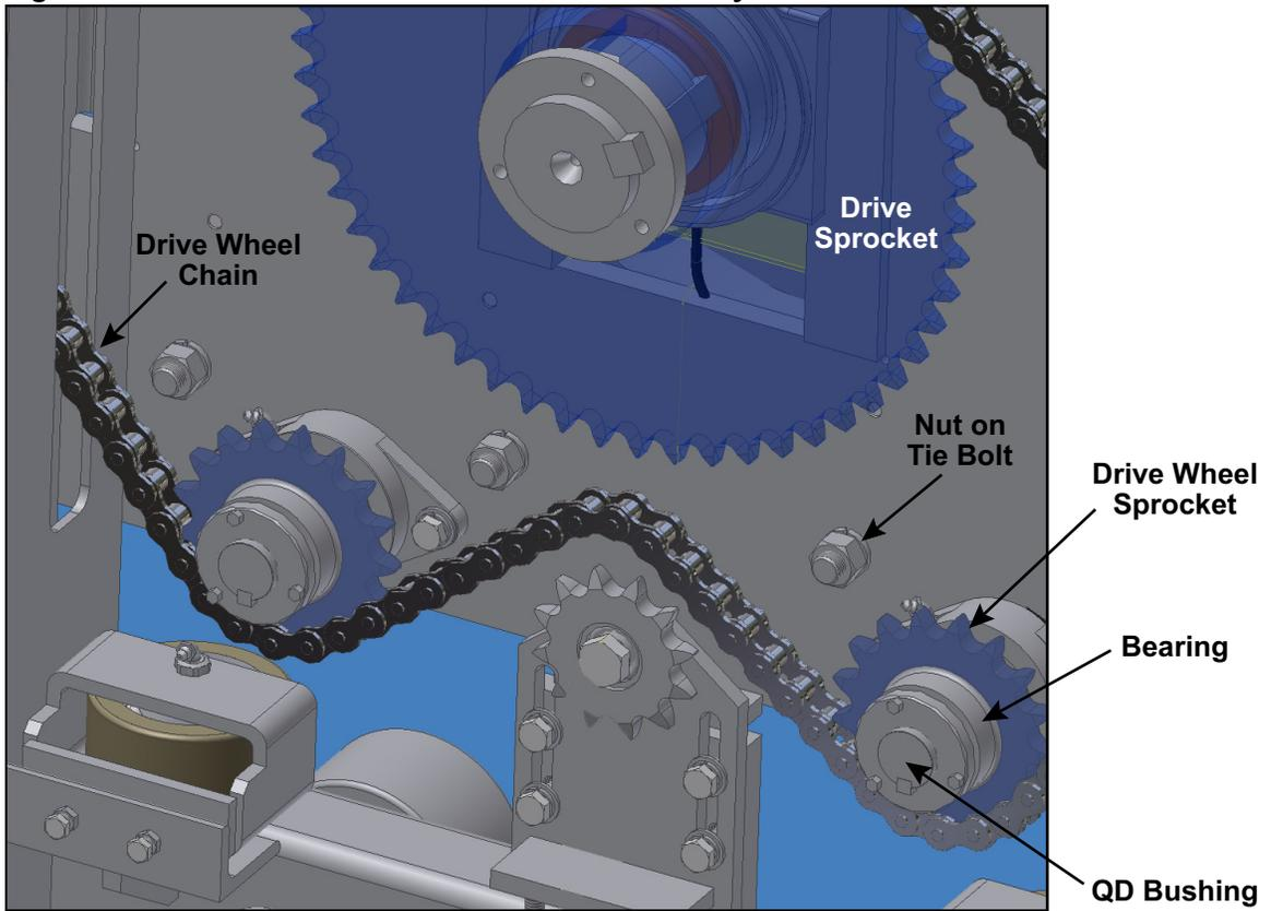
**Figure 6-10: Drive Wheel Block on Inner Side of Gantry Head**
