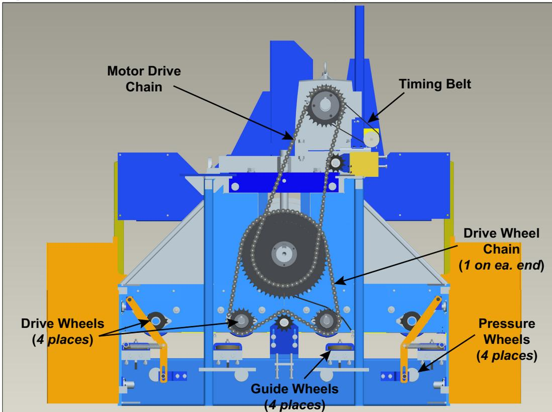
Figure 6-28: Bearing Lubrication Points, One End of Gantry Head
