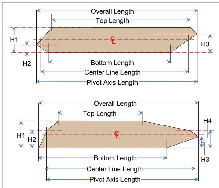
Figure 1-4: Parts of a Truss
