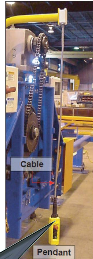
**NOTE:** When you release a directional button, the gantry head decelerates and eventually comes to a complete stop.
