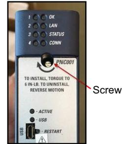
2. Note the location of each cable attached, and unplug all cables from the profinet module.
