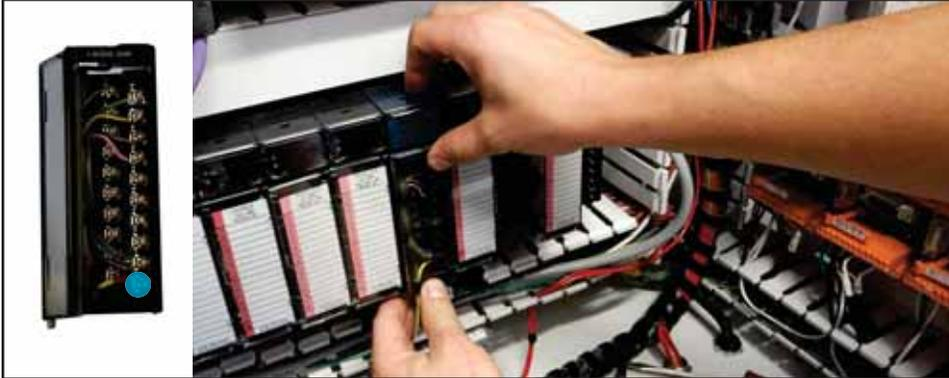
3. Route the cable through the wire duct to the interface modules. Loop any slack in the vertical wire duct on the right-hand side.
