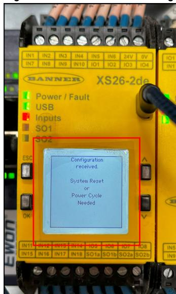
31. Power cycle the machine using the disconnect switch on the electrical enclosure.
