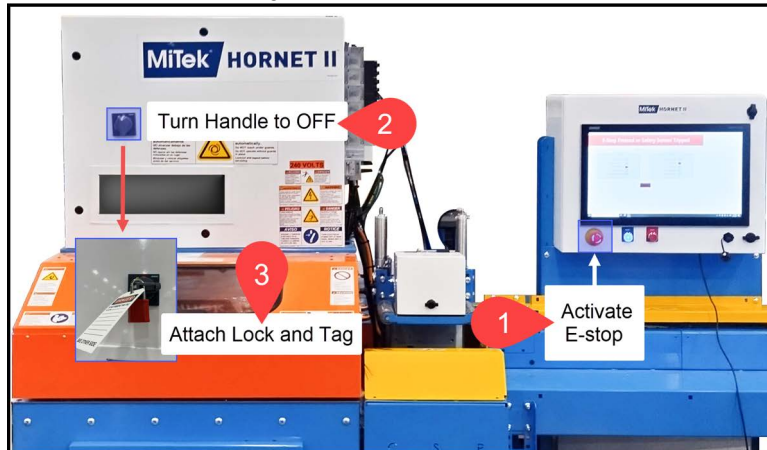
Figure 1: Disconnect Switch
