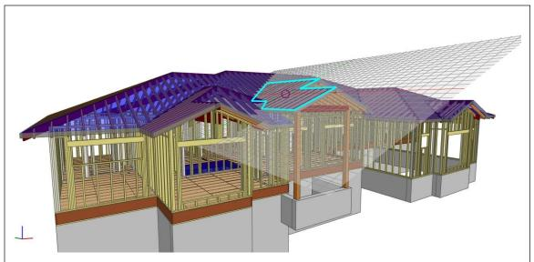
Shorter framing cycle times are realized through collaboration enabled in part by MiTek's SAPPHIRE® 3D BIM structural models (sample shown), ENTEKRA's engineered integration, and manufacturing that uses MiTek automated equipment.
